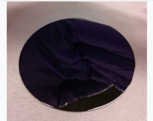
GaAs wafer of (100) orientation
